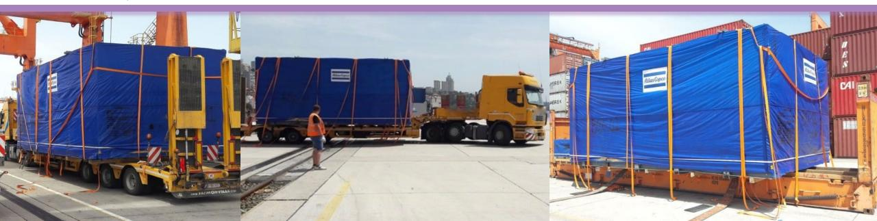
8x OOG Generators and turbines, biggest piece was over 10 meter long, just under 5 meter wide and 4 meters high and reaching almost 100 tons
