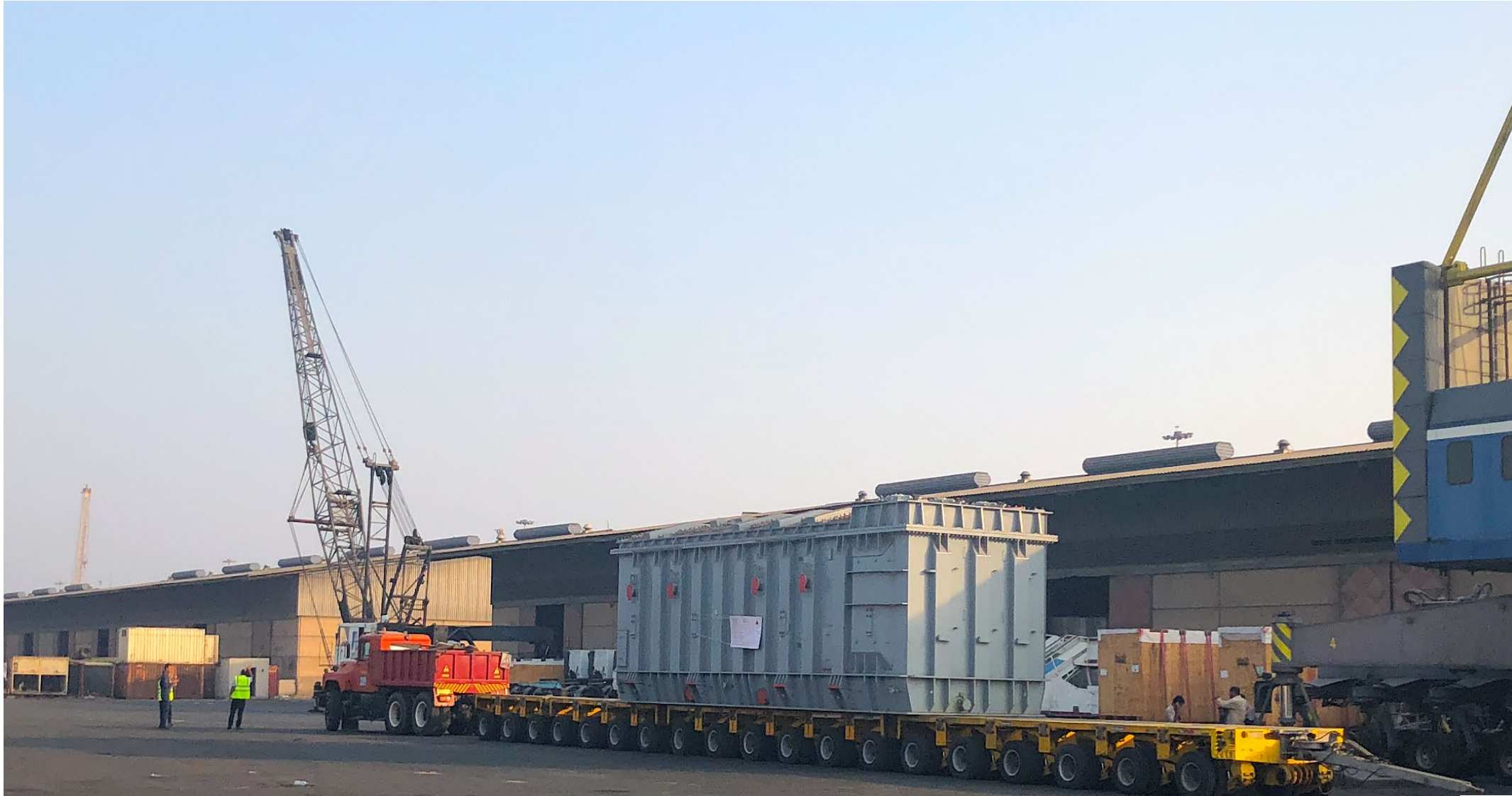
Transportation of 2 x 320 tons Transformers
