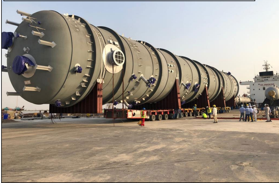
VDU – 520 tons (54 x 11 x 10 (LxWxH) in meter)
