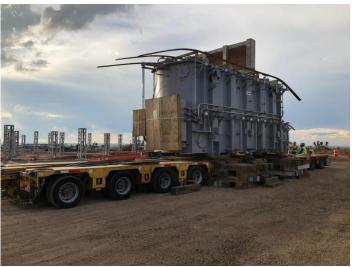
114 TONS per transformer Total weight: 406.56 TONS
